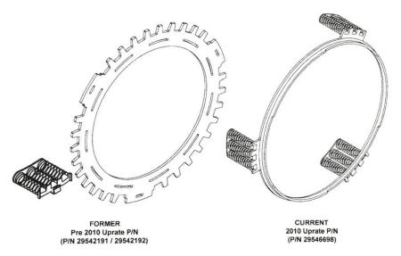
When updating the C3/C4 clutch sections to the later LML style setup, you will also need to install the four .079" thick C3/C4 steel reaction plates (29546701-079-X) included in this kit.
